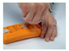
3. At its stop position press the lid with gentle pressure further toward. The lid jumps out of its anchoring and you hear a slight click.
